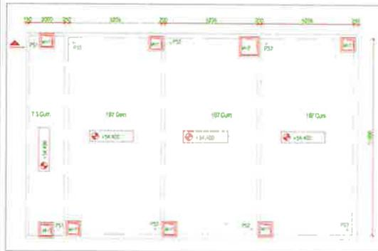
RAIN WATER SUMP AT COVER SLAB LEVEL WITH PUMP DETAILS
